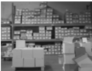
Conventional IR camera with ordinary lens shifts the image focus under IR illumination
